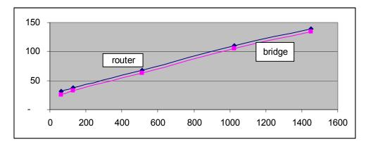
Figure 13. Linux Router Latency Test (Latency in µs vs. Frame Size)
